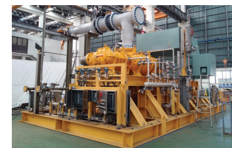
Propane Refrigeration Compressor - Korea 4032XLLLC / 3000kW
