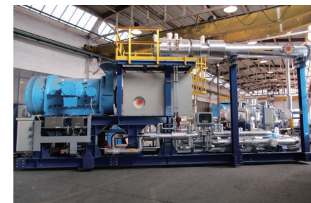
PSA Compressor - Russia 400L / 1320kW
